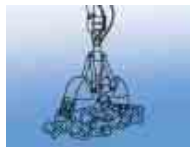
The clamshell grab allows easy positioning, and grabbing of sea bottom deposits, especially through a limited opening of excavation.
