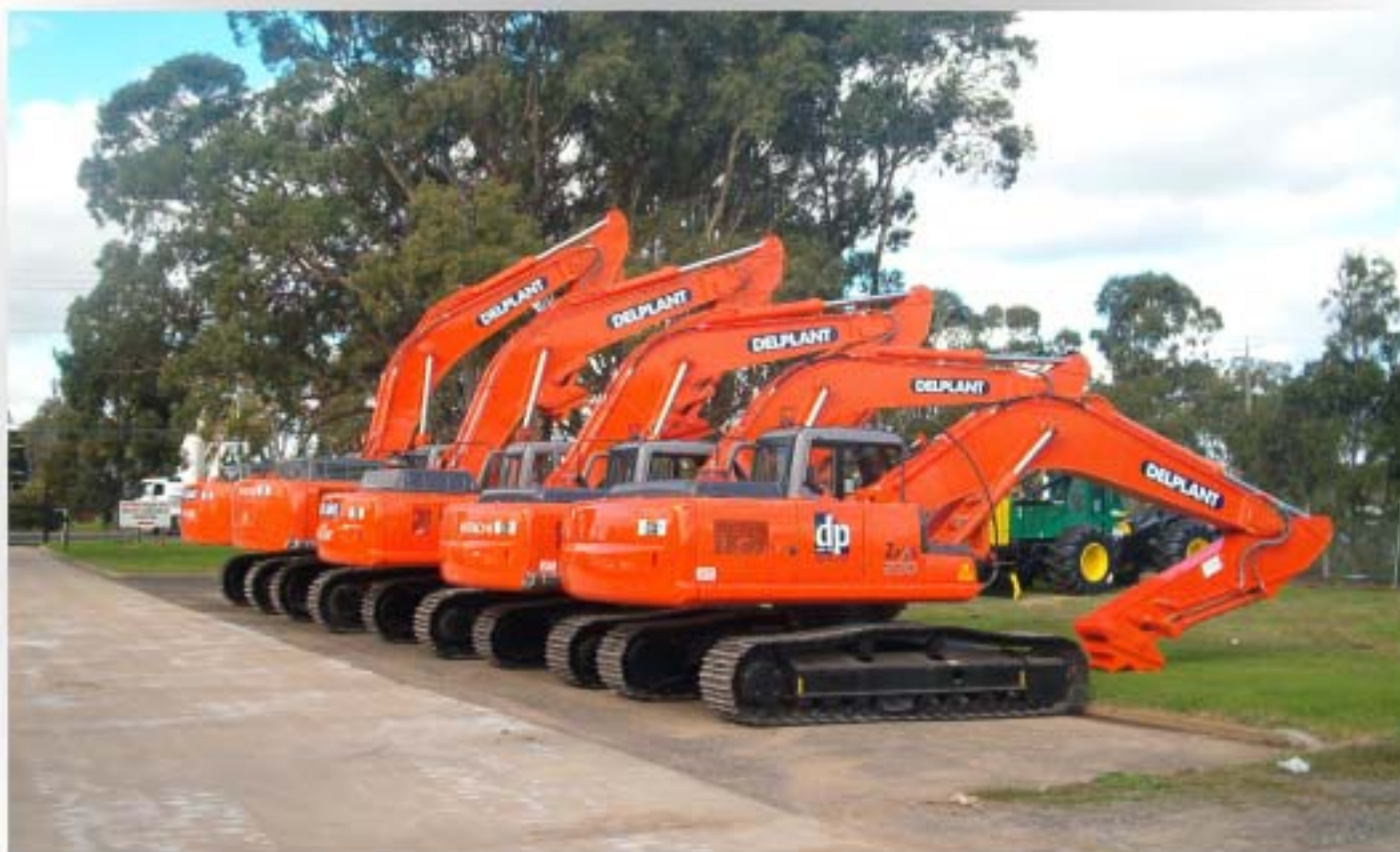
The latest additions to the Delplant equipment fleet – two 23-tonne Zaxis 230s, a 32-tonne Zaxis 330 and two 44-tonne Zaxis 450s – will be used primarily on pipeline contracts or as hire machines.
